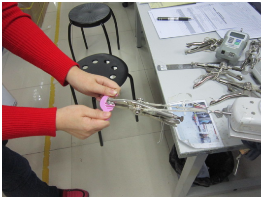
Image 1 (Clamp with 19 mm discs) Force applied parallel to teeth
